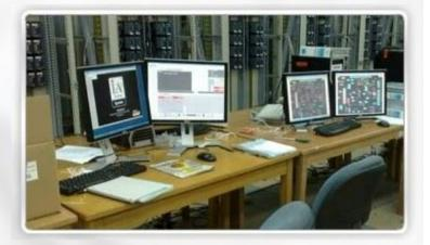
**DCS:** These control systems are hardware and software systems that distribute important control functions, for example, controllers, historians, and display units or human-machine interfaces (HMIs), into different boxes. Today, most process industries, such as oil refineries, chemical plants, and paper-making plants, use DCS.
